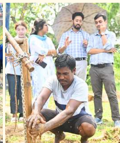
Some glimpses from the demo class and field demonstration of SPT to determine the safe bearing capacity (SBC) of the soil and eventually the depth of foundation.
