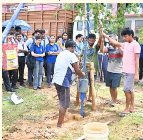
Some glimpses from the demo class and field demonstration of SPT to determine the safe bearing capacity (SBC) of the soil and eventually the depth of foundation.
