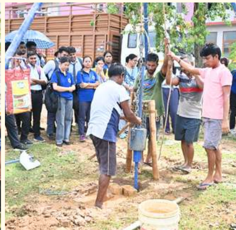
Some glimpses from the demo class and field demonstration of SPT to determine the safe bearing capacity (SBC) of the soil and eventually the depth of foundation.
